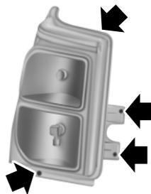
7. Remove the four bolts from the headlamp assembly.
