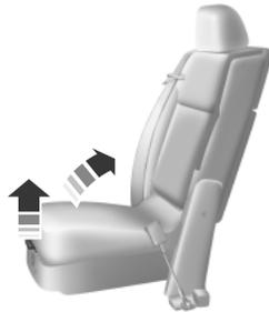
To gain access to the under-seat storage compartment (if equipped) in your seat cushion, lift the latch to open the lid. The lid cannot be opened when the armrest is down.
