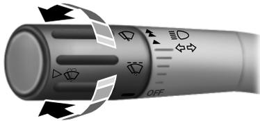
Rotate the end of the control away from you to increase the speed of the wipers. Rotate toward you to decrease the speed of the wipers.
