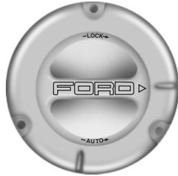
For proper operation, make sure that each hub is fully engaged and that both hub locks are set to the same position (both set to LOCK or both set to AUTO). To engage LOCK, turn the hub locks completely clockwise; to engage AUTO, turn the hub locks completely counterclockwise.
