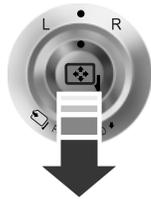
Pull the control back to fold the mirrors in or out.
