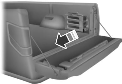
2. Open the latches to release the panels.
