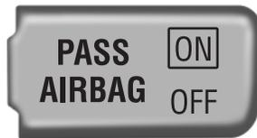
The front passenger sensing system uses a passenger airbag status indicator that will illuminate, indicating that the front passenger frontal airbag is either **ON** (enabled) or **OFF** (disabled). The indicator lamp is located by the radio.
