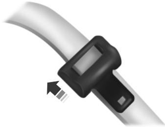
1. To lengthen the lap belt, pull some webbing out of the shoulder belt retractor.
