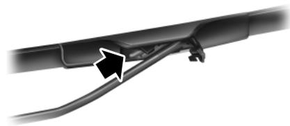
2. Press the retaining clip to disengage the wiper blade, then pull the wiper blade down (C) toward the windshield to remove it from the arm.
