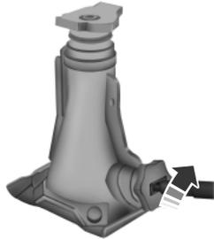
7. Turn the jack handle clockwise until the wheel is completely off the ground and high enough to install the spare tire.
