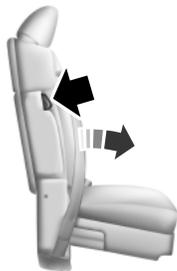
To release the armrest and gain access to the cupholders and seat back storage bin, press the button on the right-hand side of the seat and pull the seat back down.
