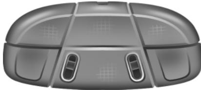
Your vehicle may have map lamps within the rear dome lamp. Press the switches on either side of the dome lamp to turn the lamps on.
