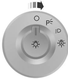
The autolamp system provides light sensitive automatic on-off control of the exterior lights normally controlled by the headlamp control.
