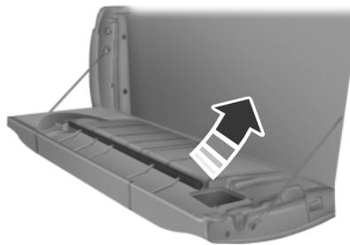
3. Raise the handle upright until you feel it latch and see the latch lever in the lock position. The yellow lever only needs to be used when releasing the grab handle.
