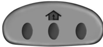
The universal garage door opener replaces the common hand-held garage door opener with a three-button transmitter that is integrated into the driver's sun visor.
