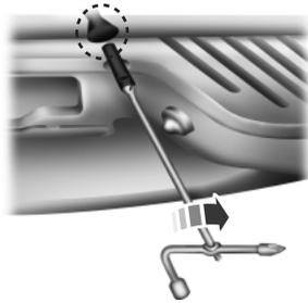
3. Fully insert the jack handle (with one extension) through the bumper hole and into the guide tube. The key and lock will engage with a slight push and counterclockwise turn. Some resistance will be felt when turning the jack handle assembly.
