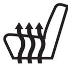
Press the heated seat button/symbol to cycle through the various heat settings and off. Warmer settings are indicated by more indicator lights.
