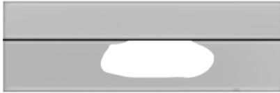
4. On the wall or screen you will observe a light pattern with a distinct horizontal edge towards the right. If this edge is not at the horizontal reference line, the beam will need to be adjusted so the edge is at the same height as the horizontal reference line.
