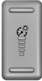
Use to adjust the brightness of the instrument panel and all applicable lit components in the vehicle during headlamp and parking lamp operation.
