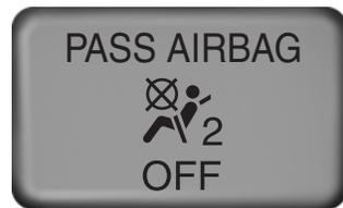
The front passenger sensing system uses a pass airbag off indicator which will illuminate and stay lit to remind you that the front passenger frontal airbag is disabled. The indicator lamp is located by the radio.
