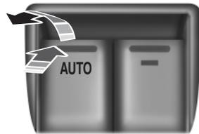
Press the switch to open the window.
